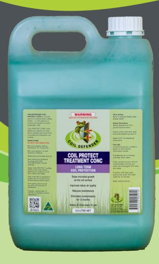
Coil Protect Concentrate is mixed with acetone or ethanol 1: 4. This is an antimicrobial treatment applied annually as a thin coating to indoor HVAC and refrigeration coils to stop bacteria, mould and slime from colonising the coil.
